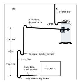
3. Piping should be designed with adequate three-dimensional flexibility to avoid excess vibration. It should not be in contact with the surrounding structure, unless a proper tubing
