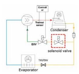
An additional solenoid valve has to be installed, it should close when compressor stops to prevent from liquid slug.
